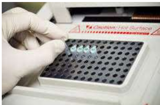
Figure 7.40:. A PCR machine showing the wells where the PCR tubes are inserted
